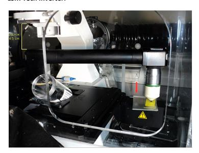
The current version installed on our microscope has a long arm meant to position the objective off to the side of the stage. Perhaps a better configuration for us would be a tube to lift the objective higher and a shorter arm to position the objective over the current stage. We need to make better measurements, but essentially the following picture.
